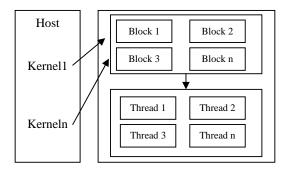
Fig. 4. GPU programming model
